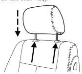
Properly adjust the head restraint so that the top of the head restraint is even with the top of your head and positioned as close as possible to the back of your head. For occupants of extremely tall stature, adjust the head restraint to its full up position.
